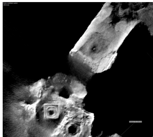
Fig. 12 Flat area with rivet at 1 o'clock. ©2005 Antikythera Mechanism Research Project. All rights reserved.
