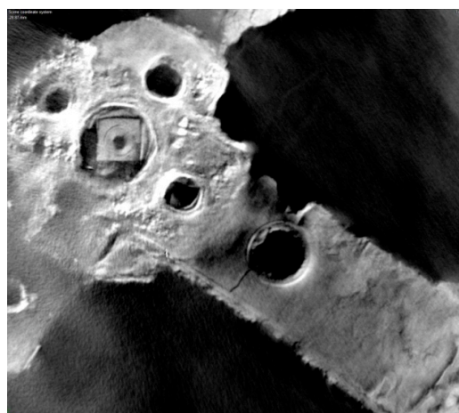
Fig. 13 Apparent bearing in the 4 o'clock position. ©2005 Antikythera Mechanism Research Project. All rights reserved.
